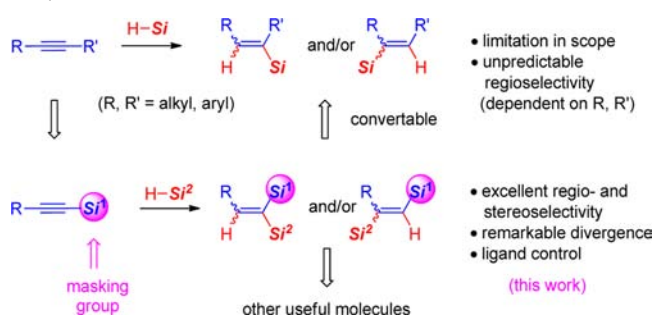
Scheme 1. Design of Intermolecular Hydrosilylation of Silyl Alkynes
